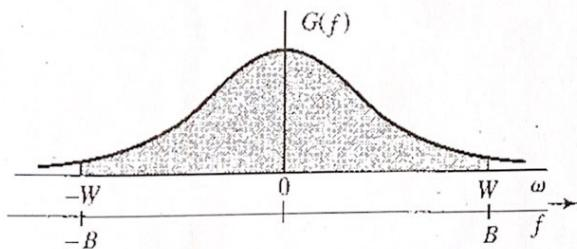
This ESD is shown in Fig. 3.33. Moreover, the signal energy  $E_g$  is the area under this ESD, which has already been found to be  $1/2a$ . Let  $W$  rad/s be the essential bandwidth, which contains 95% of the total signal energy  $E_g$ . This means  $1/2\pi$  times the shaded area in Fig. 3.33 is  $0.95/2a$ , that is,
