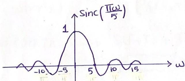
Nulls @  $\omega = \frac{\pi\omega}{5} = \pm\pi, \pm 2\pi, \pm 3\pi, \dots, (\pm n\pi)$
