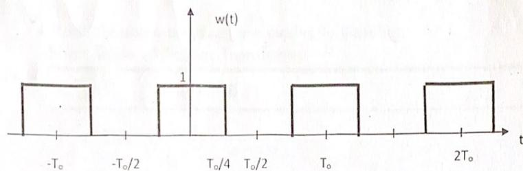
2. For the following periodic signal, find the exponential Fourier series, then sketch the amplitude and phase spectra.
