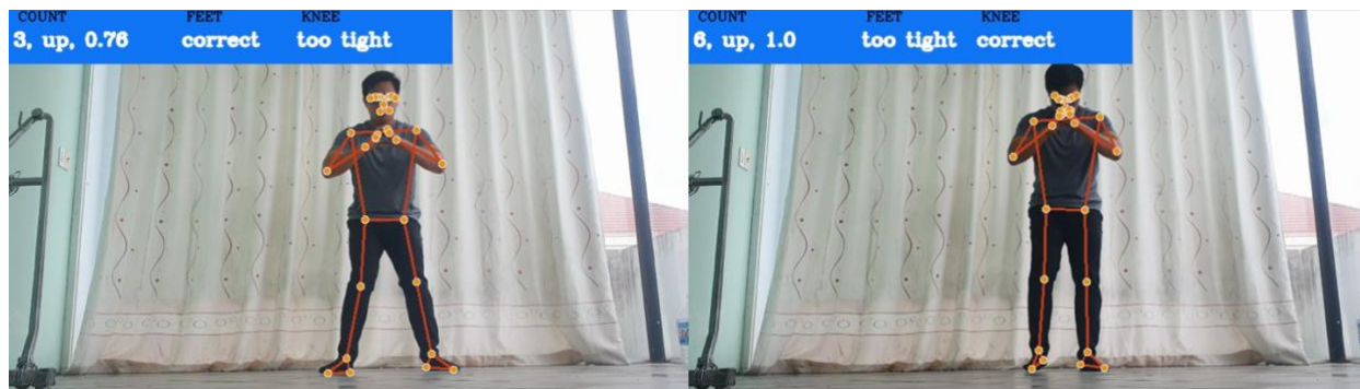
Figure 27: Test QB-03. Squat error detection
