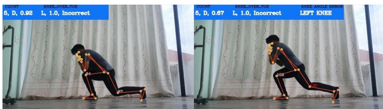
Figure 28: Test QB-04. Lunge error detection
