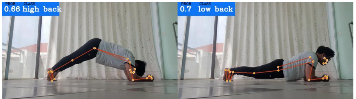
Figure 26: Test QB-02. Plank error detection
