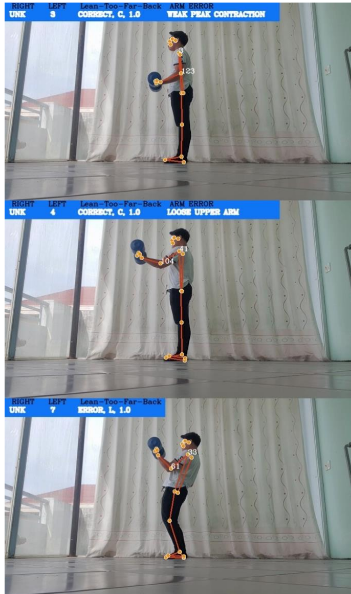
Figure 25: Test QB-01. Bicep Curl error detection
