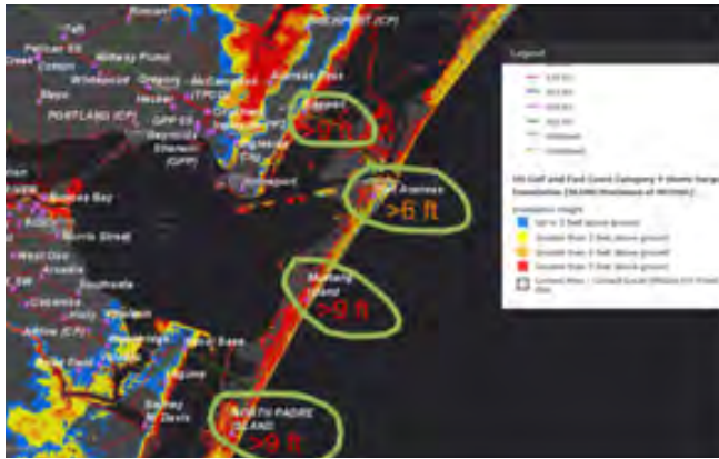
Category 4 hurricane storm surge map for part of the coastal area of Corpus Christi, Texas. The areas circled reflect the locations of four substations and the level of storm surge to which they could be exposed.
