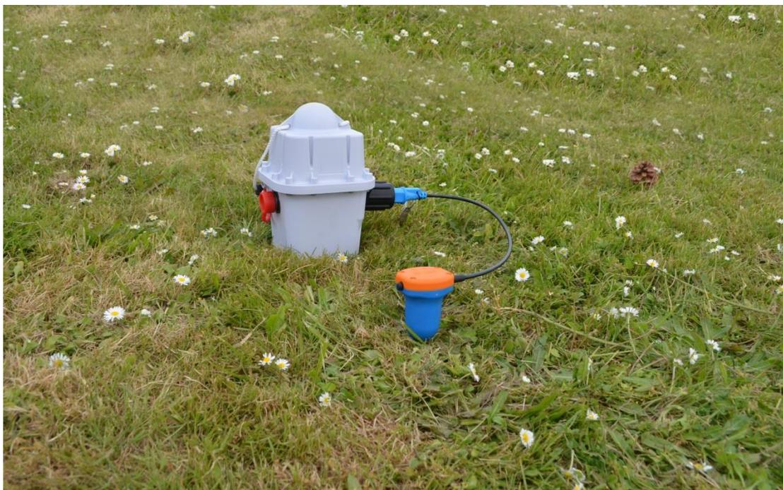
*Sercel SG-5 single sensor connected to the UNITE node RAUeX (image courtesy of Sercel).*
