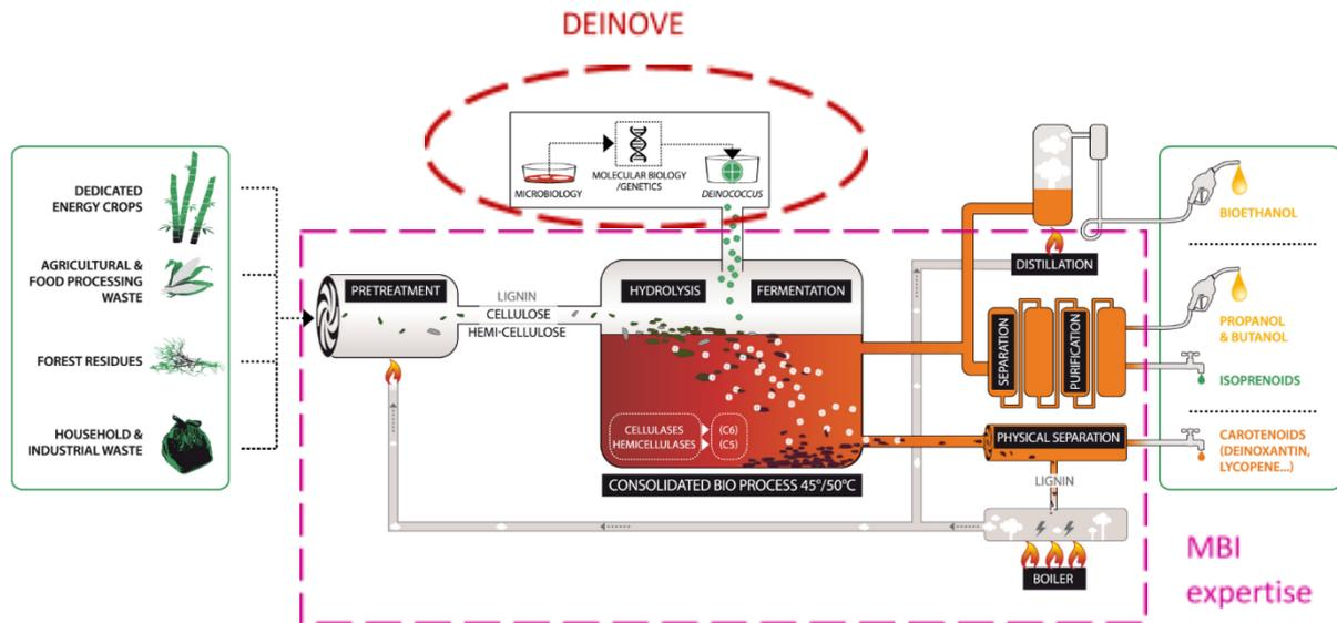
DEINOL is a production system aimed at converting pretreated industrial biomass into ethanol. The DEINOL solution’s major industrial interest lies in the ability of *Deinococcus* bacteria to break down the complex sugars contained in lignocellulosic biomass and then to convert them into ethanol, all in a single operation, replacing the microorganisms that are traditionally used and a large part of the enzyme treatment that precedes fermentation.
